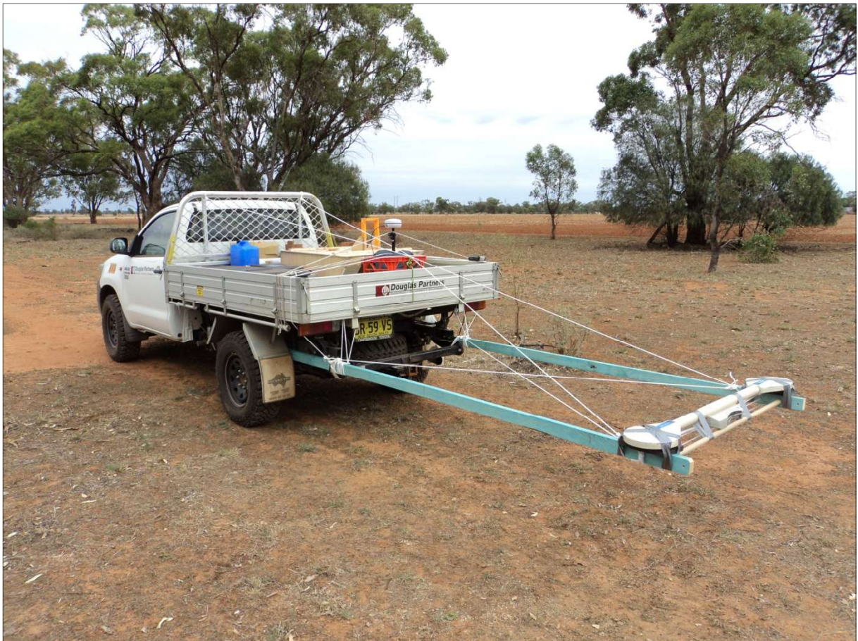
Figure 2: Profiler on booms behind a 4WD (not this project) and DGPS antenna in tray of 4WD.
